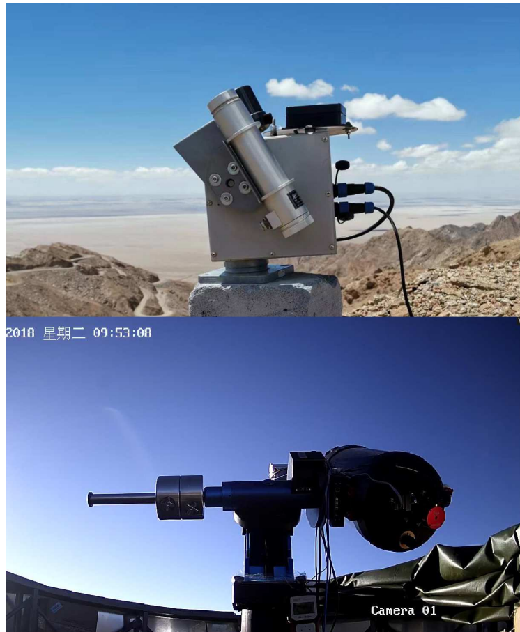
Fig. 8: The solar direct radiation meter was mounted on a fully automatic Solar tracker in Mt. Saishiteng (top). The field of view of solar radiation meter is 5^\circ and tracking accuracy of solar tracker is less than 1^\circ . S-DIMM and precipitable water vapor spectrometer were mounted together on an ATR equatorial mounting at Mt. Saishiteng (bottom).
